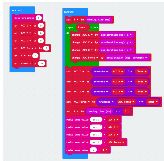
Figure 11. Program of the Transmitter micro:bit
